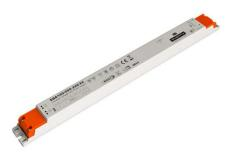
Features: .Built-in constant voltage LED driver .Built in push dimming .Comply to DALI 2.0 standard(IEC 62386-101,102,207) .Linear or log curve optional .Dimming range 1.0-100% .Start-up time is less than 0.5s .Open circuit, short circuit, overload, over temperature protectior .Efficiency greater than 92% .For indoor lighting,office lighting .5 years warranty
